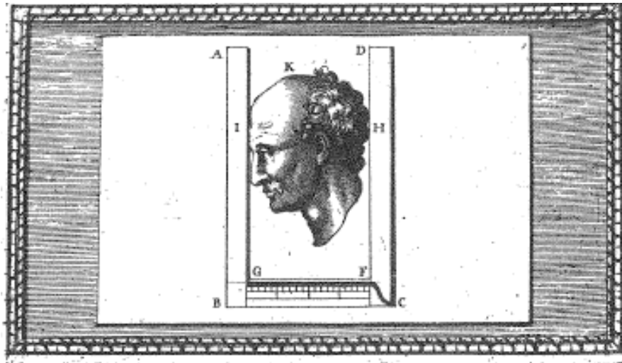
Fig. 7.2 Illustration depicting Alberti's use of two set squares— normae —which was used to measure both the length, width and breadth in the exempeda system (Source: Gadol 1969, 77.)
